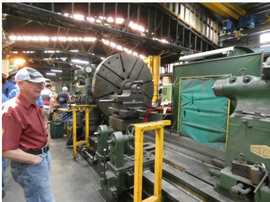
Mel' Norton inspecting a large faceplate lathe inside the workshops
