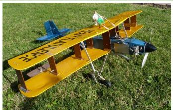
An unusual model, called "Heavy Flatulence "Heavy, as the whole thing is made from 3 ply, Flat as the wings have a flat profile, the Ulence refers to the motor exhaust piped to the rear of the model, O.S 46 LA power, plus many other unusual features, should be fun
