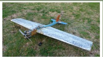
This is a control line trainer, called a UKI, it has a foam wing, elevator control only, 46 LA power, stick fuselage, all ready to go
