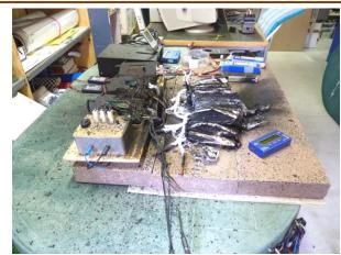
These LiPOs were incinerated, the workshop survived because the fire did not spread ,due to the fireproof surface under the LiPOs ( concrete pavers ), I now include small cash boxes to enclose the LiPOs, ( from Bunnings )
