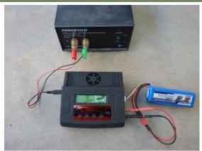
A typical computer controlled charger, and power supply, on a fire safe concrete surface
