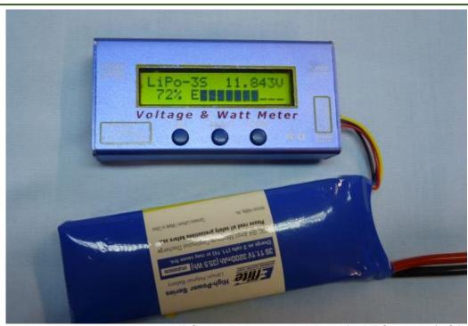
A typical battery tester, set to test a LiPO, the display shows, it is set for LiPO, 3 cells ( 3S ) The voltage is 11.8 volts
