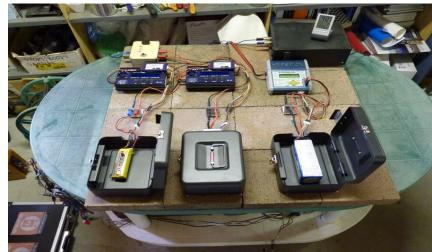
A LiPO charging set-up on concrete pavers, for extra fire protection the LiPOs are placed in the little metal cash boxes, (from Bunnings)
