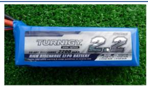
A typical LiPO battery 2.2 amp hour, 3 cell, 11.1 volts
