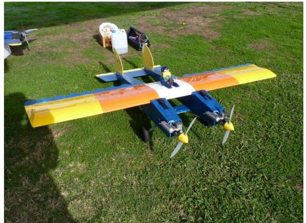
Wally Schubach's ill fated twin boom apparatus, it was seriously lacking elevator authority
