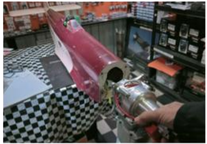
Quarter scale Miles Hawk Speed Six with the ubiquitous Desert Aircraft DA 85 engine
