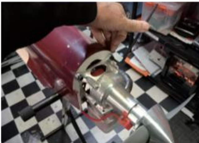
Quarter scale Miles Hawk Speed Six with the ubiquitous Desert Aircraft DA 85 engine
