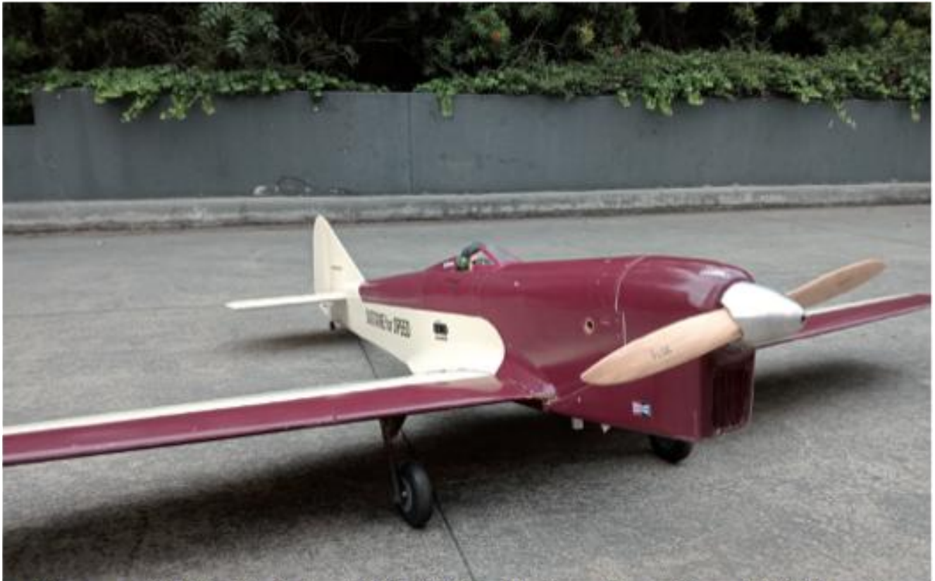
Quarter scale Miles Hawk Speed Six with the ubiquitous Desert Aircraft DA 85 engine
