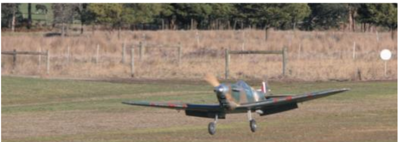
Centre of Gravity sorted at last - Stable approach with 2mm up elevator mixed and forty five degrees of split flap
