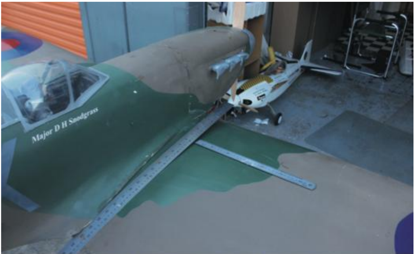
Tank empty, gear down the CofG is 195mm from the leading edge. Up elevator measured at its widest point is 35mm - 39 mm down, This produces a good flying experience
