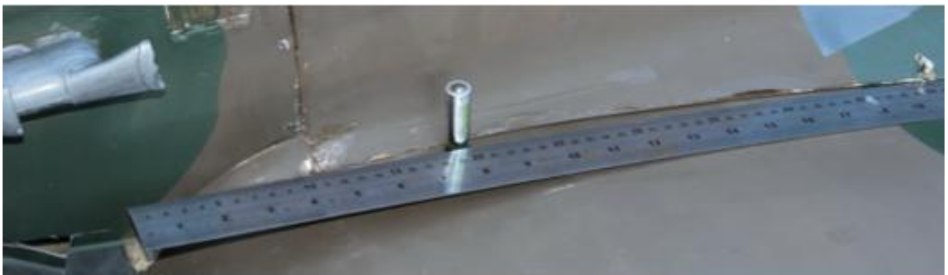
Chord at this location is 570 mm. 195\text{mm} / 570\text{ mm} = 34\%
