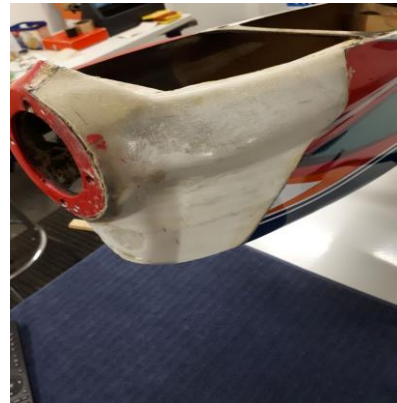
Fiberglass repair under way
